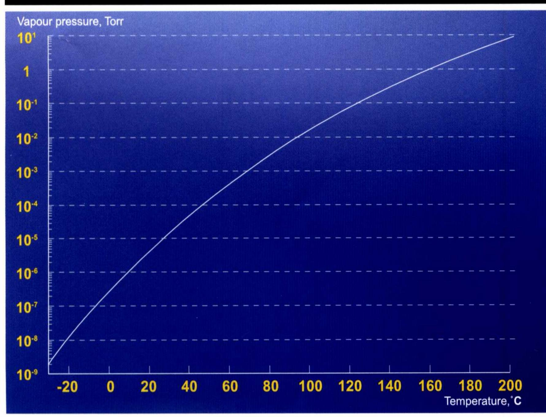
Apiezon AP201 was developed over 20 years ago specifically for use in vapour booster pumps to replace oils based on PCBs.
